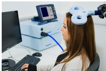
Figure 1 TMS example. In this instance a figure-of-eight coil is used during a behavioural experiment. The TMS readout is so called electromyography (EMG), which monitors muscle activity.
